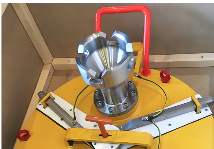
Hatch with integrated stab receptacle and electrical strapping for long term service
