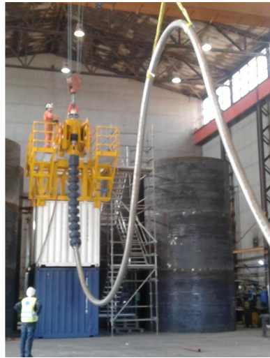
Illustration of intervention hose with weak link during testing prior to delivery
