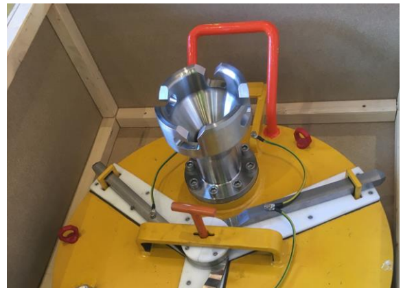
Hatch with integrated stab receptacle
