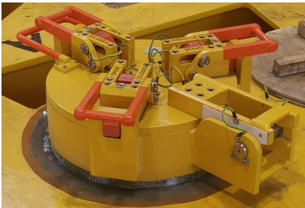
Hatch with electrical strapping for long term service
