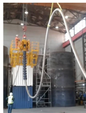
Illustration of intervention hose with weak link during testing prior to delivery
