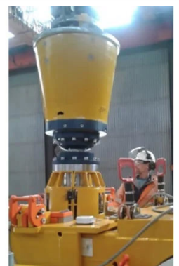
Illustration of intervention hose with weak link during testing prior to delivery
